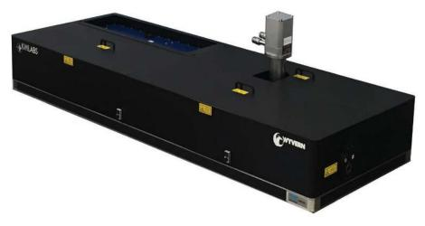
Wyvern-1000™ is KMLabs' sub-40 fs, single-stage regenerative amplifier. It is a fully engineered and integrated commercial source based on a single rugged opto-mechanical platform. It employs patented (US 6,804,287) cryogenically-cooled amplifier technology, allowing for a continuous trade-off between pulse energy and repetition rate.
