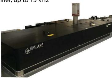
Dragon<sup>™</sup> is KMLabs' sub-25 fs, single-stage multipass amplifier. It is a fully engineered and integrated commercial source based on a single rugged opto-mechanical platform. It employs patented (US 6,804,287) cryogenically-cooled amplifier technology, allowing for a continuous trade-off between pulse energy and repetition rate.
